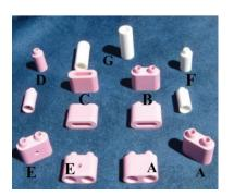
These special sintered alumina ceramic beads can be used for preheating and postheating of welding applications because of their excellent heat resistance.
